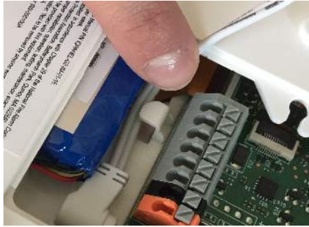
Route the wire behind the retainer clip
