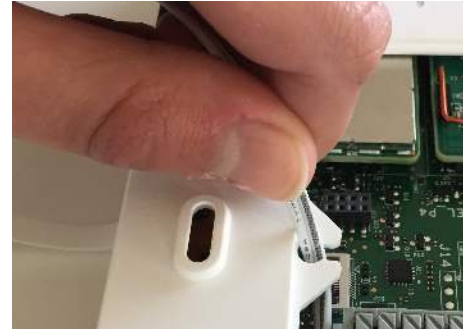
Insert the wire into the strain-relief
